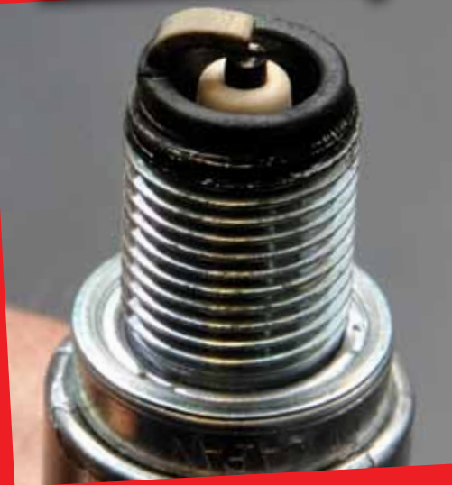
To confirm the dyno air-fuel ratios, spark plugs were removed. Though the heat mark on the ground strap is not clearly visible in this photo, the color change is almost mid-way, suggesting correct ignition timing. The porcelain also reveals healthy color and there is no evidence of soot deposits on the base ring, which indicates correct jetting. LWA aims for one to two blackened threads on a street engine; on a race motor that generates more heat they aim for two to three blackened threads and a slightly lighter color on the base ring.
